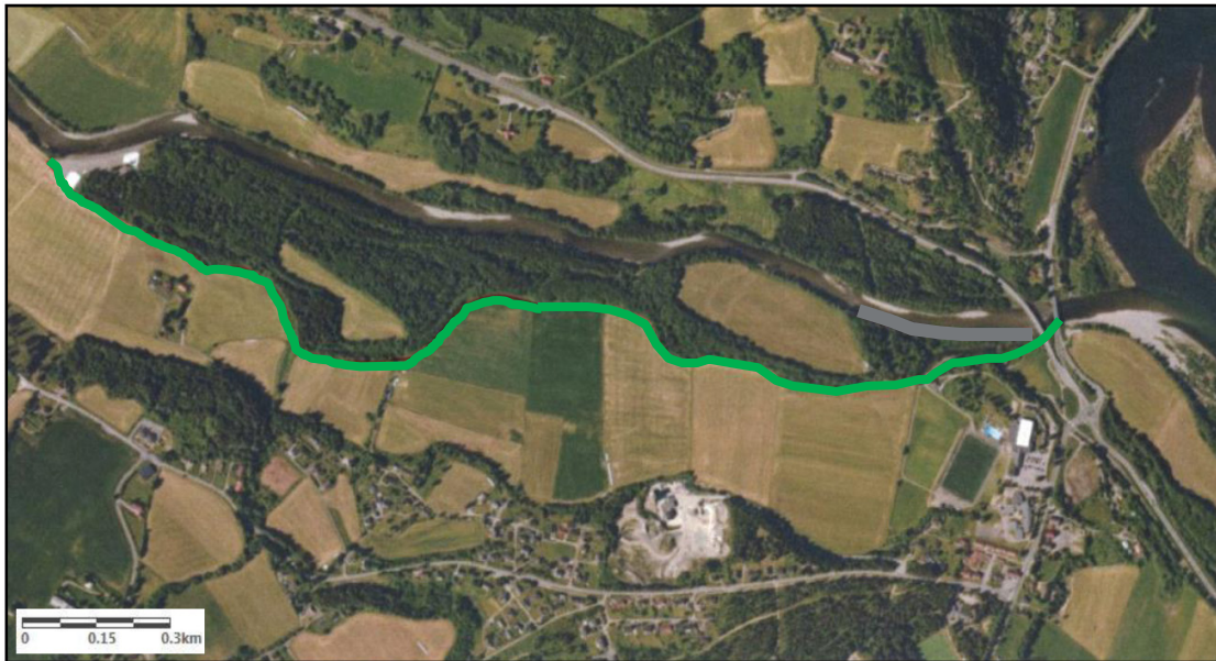
Figure 3.1 The planned location of the receded flood barrier (green) at Jorekstad. The main river Lågen is seen in the right part of the picture, and the old protection, which will be removed, is shown in grey.
