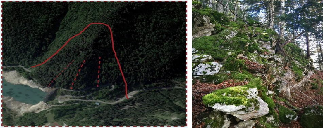
Figure 3.10 Overview of the hazardous area at Artouste (left), and one of the identified release zones for rock fall.
