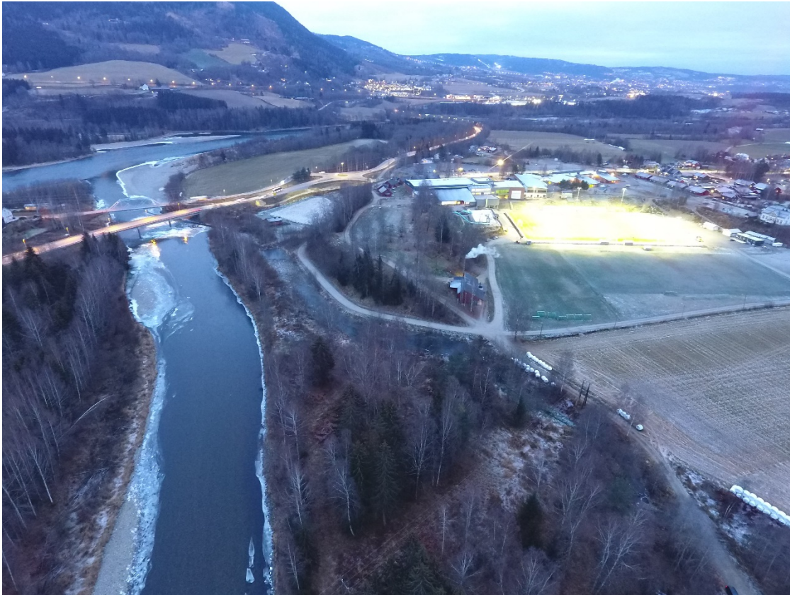
Figure 3.6 Drone photo of the outer parts of the Gausa river, where it meets the main Gudbrandsdalslågen river. The planned barrier will come in from the lower right, along the pile of white, plastic covered hay balls, and protect the sporting facilities and the buildings behind it. The city of Lillehammer in the far background. (Drone photography by Multiconsult).
