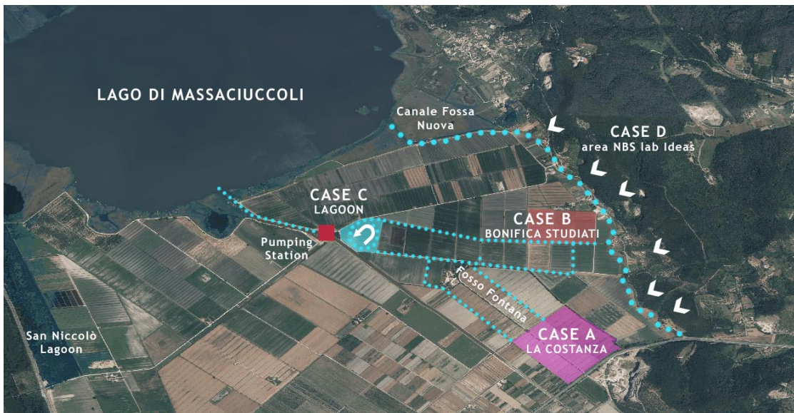
Figure 4.3 Orthophoto from 2013 showing the two areas of buffer strips (Case A and B) and the location of the retention basin (Case C). The figure also shows the main Fossa Nuova canal, to which the diversion pipeline will lead water from the Serchio River during dry periods. Case D in the hills to the east, marks the third proposal (below).
