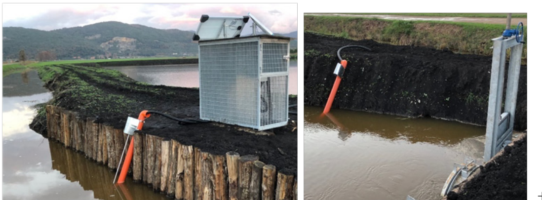
Figure 4-15 Photos of the monitoring probes at the intake and outtake of the sedimentation basin. Their locations are marked in Figure 4-5 (Photo: ADBS)
