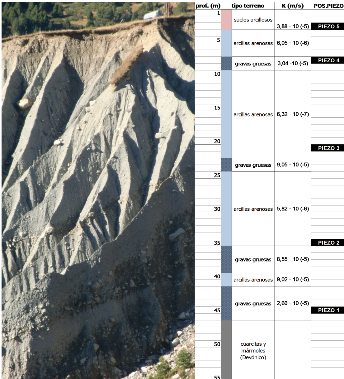
Figure 5-15 The complete till section at the Erill-la-Vall site, with stratigraphy and position of piezometers (figure by C. Raïmat).
