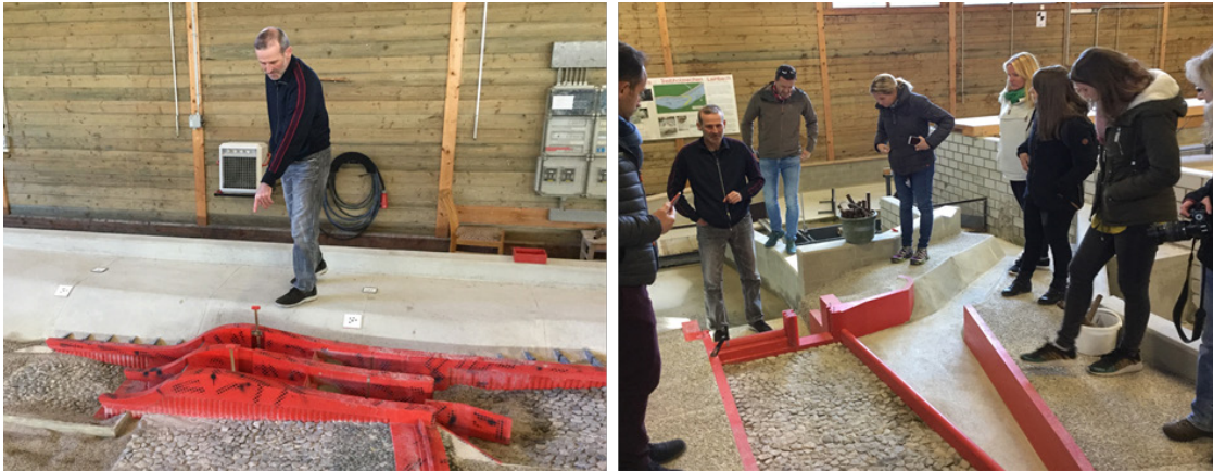
Figure 7-3 Visit to the hydraulic test facility, where all measures to be implemented were tested hydraulically in down-scaled models.
