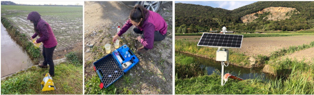
Figure 4-12 Manual periodic sampling (left) and continuous, automatic monitoring system (right) (Photo: ADBS)
