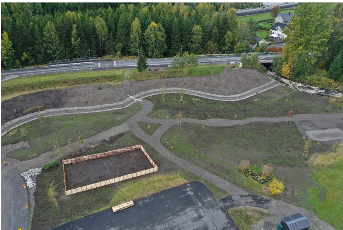
Figure 6-5 Drone photos of the Trodalen site after completion of the interventions, but before planting is fully completed. Upper: Overview of the whole intervention. Lower: The lower part, below the houses, where Trobekken ends in Søre Brynsåa. One of the two fenced-in test fields for plants in the lower foreground. These were still not in place when the upper photo was taken. (Photos by Øyer municipality).
