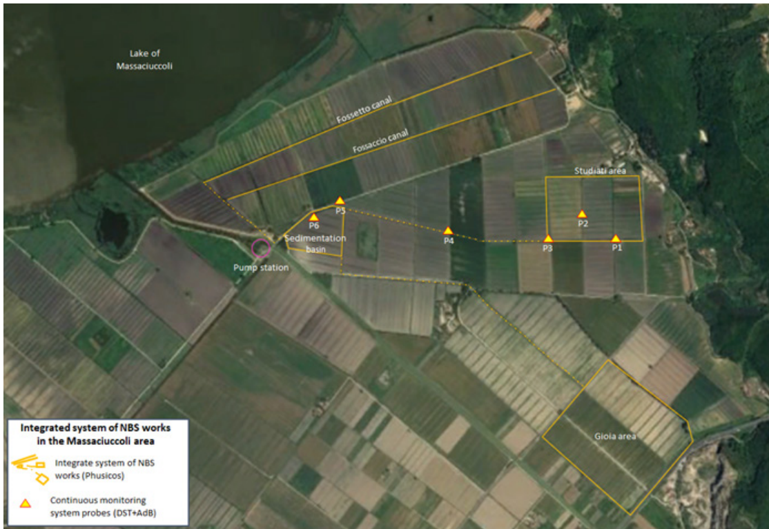
Figure 4-14 Overview of probes (yellow triangles) for automatic, continuous monitoring Of surface water parameters in the study area.
