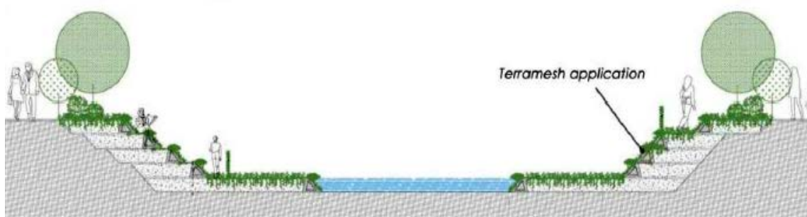
Figure C.36 Sample section of terramesh system for watercourse naturalization
