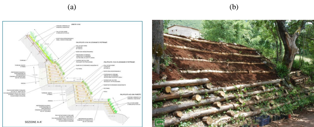
Figure C.23 Schematic description (a) and example (b) of vegetated timber cribs
