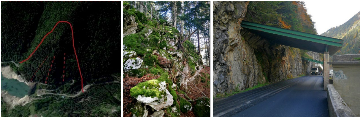
Figure 11. left) study area; center) rockfall release area; right) existing rockfall defences (rockfall tunnel).
