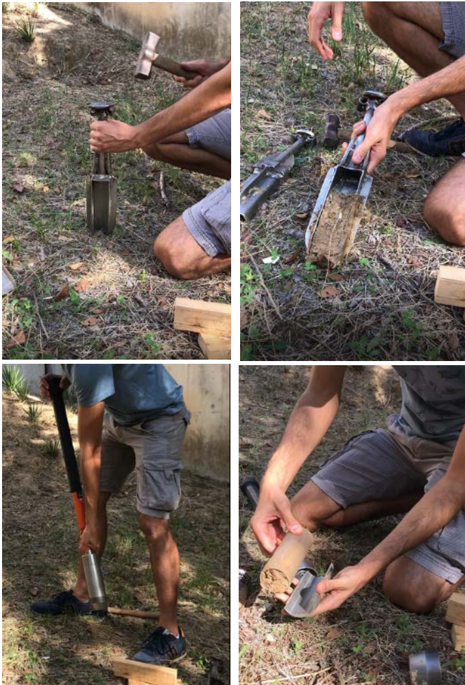
Figure 3. Soil sampling with two different types of soil corers of squared (5 x 5 cm side) or circular (5 cm diameter) section 15 cm long. Both types of corers can be opened lengthwise to obtain undisturbed soil samples of constant known volume.
