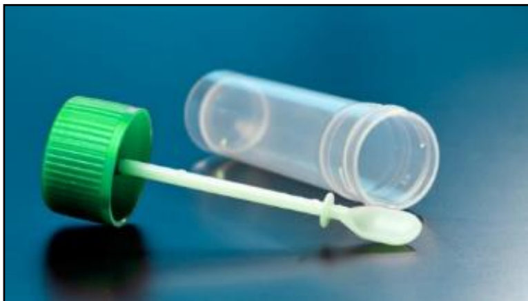
Figure 6. Sampling kit (sterile spoon and container) for soil samples allocated to microbial DNA analyses.
