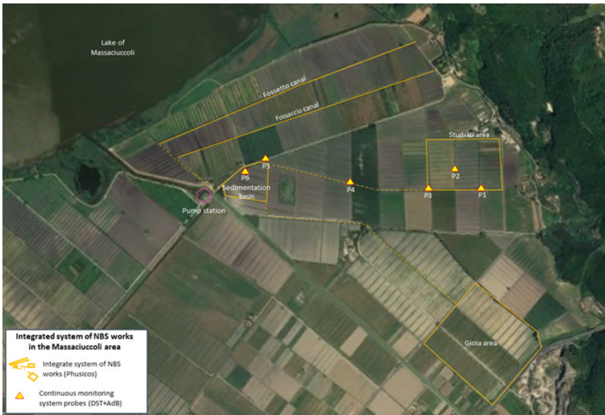
Figure 5. Overview of probes for automatic, continuous monitoring surface water parameters.
