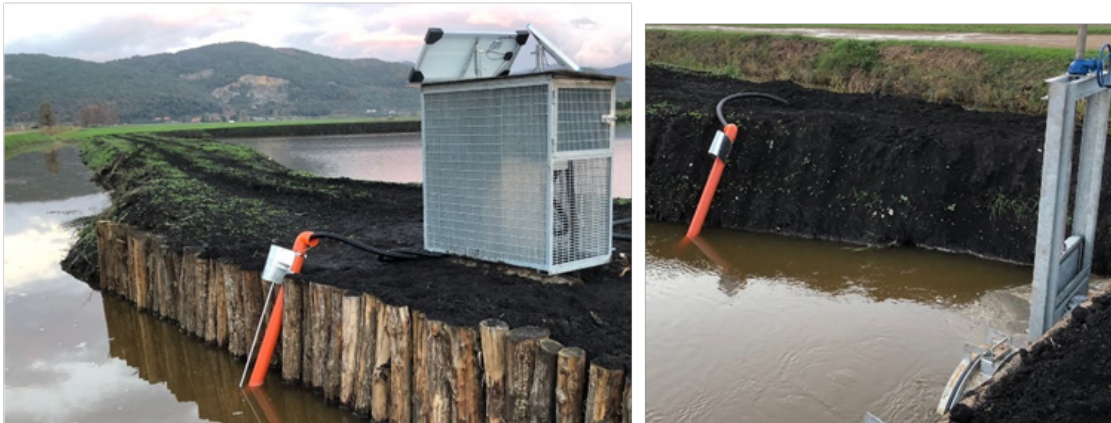
Figure 7. Photos of the two monitoring probes in the sedimentation basin (Photo credits: ADBS).
