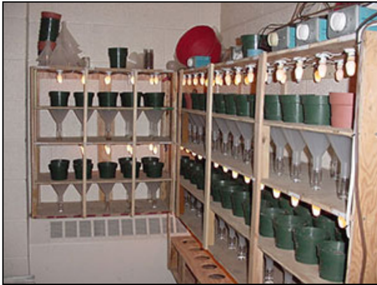
Figure 5. Berlese funnels used to extract microarthropods from undisturbed soil samples.
