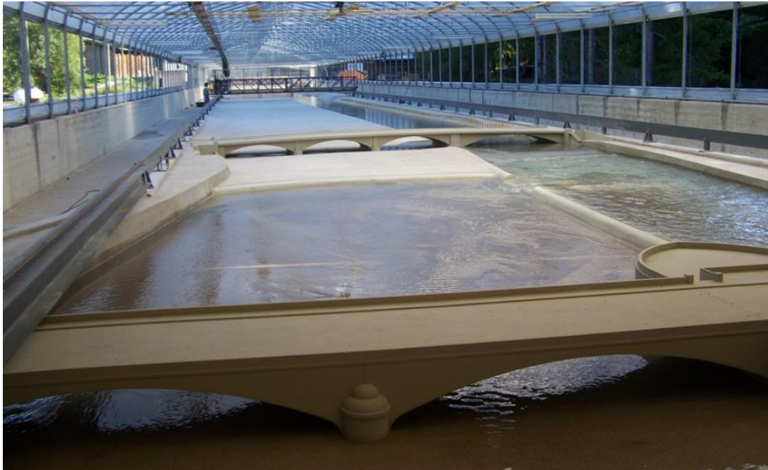
Figure 14: Experimental hydrological model of the Isar in Munich, carried out by TUM (downscaled 1:20) (Source: WWA München, n.d.)
