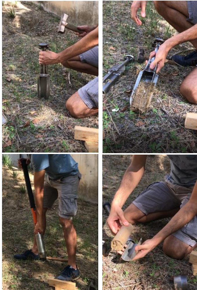
Figure 3-10. Soil sampling with two different types of soil corers of squared (5 x 5 cm side) or circular (5 cm diameter) section 15 cm long. Both types of corers can be opened lengthwise to obtain undisturbed soil samples of constant known volume.
