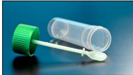
Figure 3-13. Sampling kit (sterile spoon and container) for soil samples for microbial DNA analyses.
