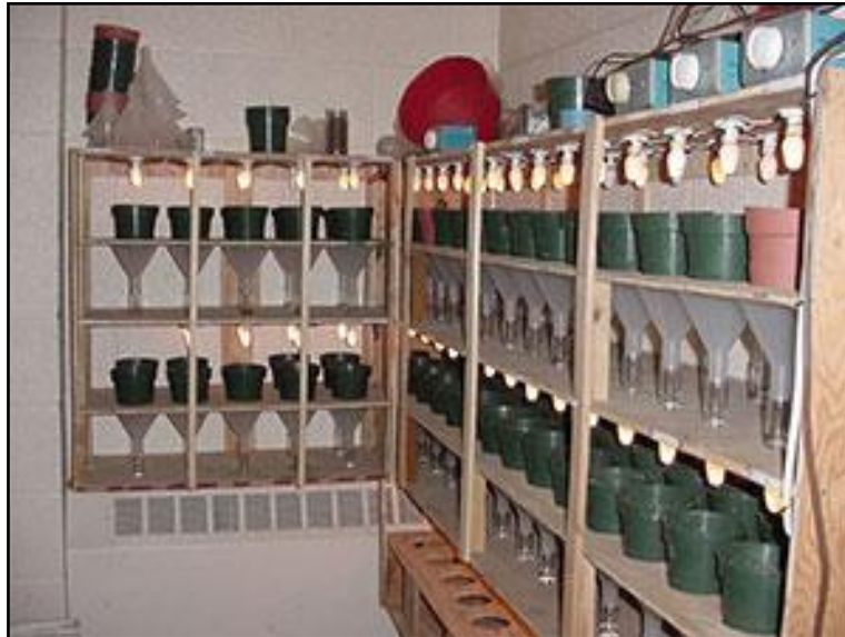
Figure 3-12. Berlese funnels used to extract microarthropods from undisturbed soil samples. Source http://soilbugs.massey.ac.nz/collection_berlese.php
